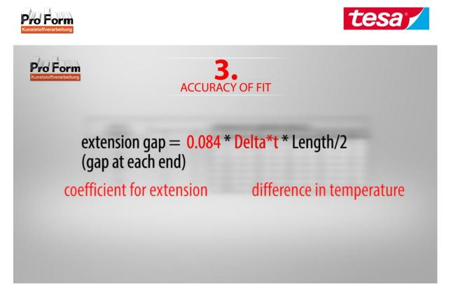
Calculate the extension gap for each end with help of the table for integration temperatures. The value **0.084** is the coefficient for extension in this formula. **Delta\*t** is the difference in temperature, of an integration temperature to the highest temperature in the summer.
