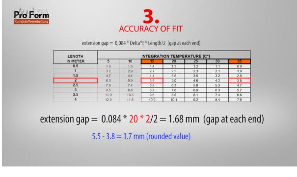
Example: As an alternative use the extension values of the table for your calculation. For our example this results in the rounded value of 1.7mm at each end.
